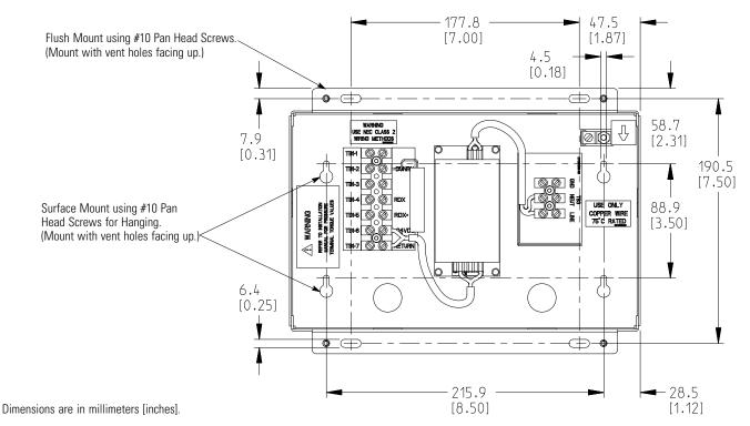
Figure 5-12. Remote Monitor Panel II Dimensions
